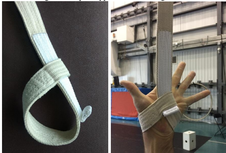
Figure 13: Stitched choke loop and position of the stitched choke loop with the hand open
