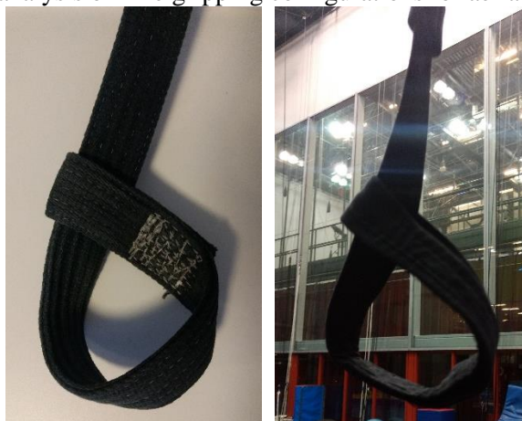
Figure 5: Strap with an integrated choke loop (stitched) and strap with loop and choke loop.
