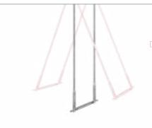
**Caution!** A sufficient surface area directly beneath the apparatus should be anticipated. There is always an angle of displacement due to acrobatic movements (controlled or uncontrolled swinging, body movements etc.).
